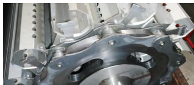
Stainless steel chain for sterilizing vegetables, frozen food, and pet food.
